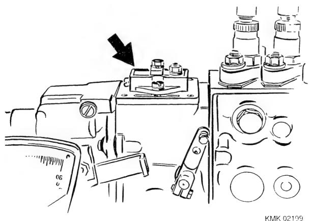
\* Lug cam with torque control
